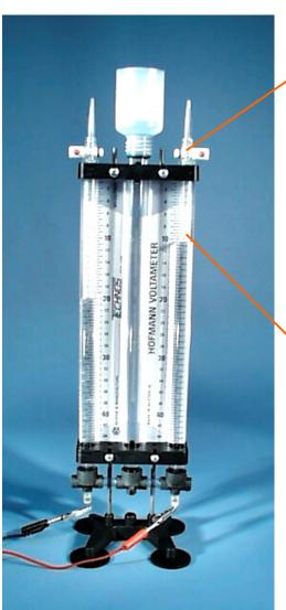
To fill the Voltameter, open both taps and, using eye protection, carefully pour the solution into the central container so that it fills the 3x tubes right up to the white plastic plug in the tap.
