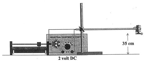
Set the rheostat so none of its resistance is included the circuit. Set the supply on 2 volt DC but do not turn it on. Check that the plastic disc on the motor shaft is horizontal and not higher than 35 cm above the level of the desk. This will ensure the ball will rotate below the eye level of a person seated.
