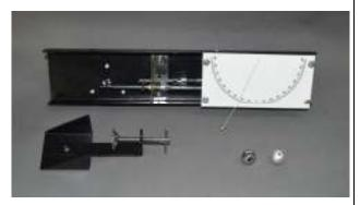
With a release latch that can be adjusted and locked in any desired setting, Supplied with two drilled balls, attached protractor and plumb bob for determination of angle of inclination. Includes a clamp to fasten the apparatus to a table top.
