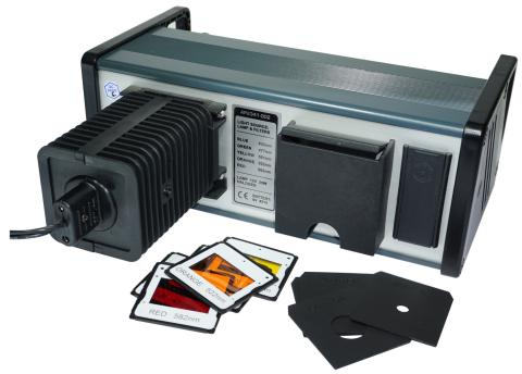
The image above shows the lamp mounted and the filters and apertures on the bench. They are normally stored in the container mounted to the panel. A small label lists the shortest wavelength (highest frequency) of light that can pass through each filter.
